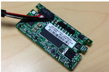
#1: CVFM04 (CacheVault Flash Module)-Front Side (to attach to the narrow end of the L3-000099 Cable Extender)
